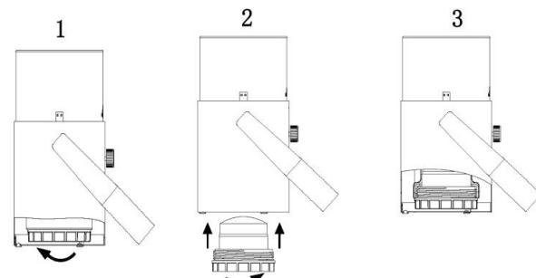
If there is a smell of gas or you suspect a leak once the cartridge has been fitted, take the appliance to a well-ventilated outdoor location away from any ignition sources. If you want to check for leaks in your appliance, do so outside. Do not try to detect leaks using a flame; use soapy water.
